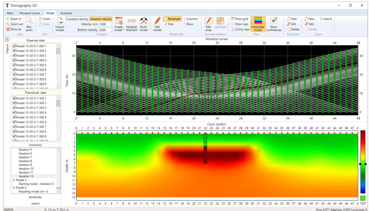
Something went wrong while tomography is calculated and you are unhappy with the ongoing values? You can pause the calculation at any iteration, change any parameters (and even the current model!) and continue. You can also scroll back through the iterations, use the result of any of them as a new initial model and start the whole process again with modified parameters.
