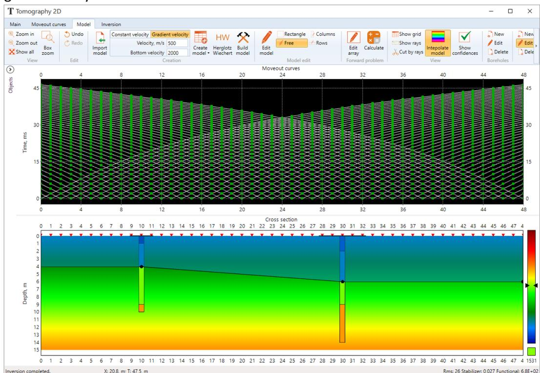
Tomography itself is based on the known Occam inversion, however with some important modification. Beside velocity, each cell of the grid has *confidence* that takes values from 0 to 1. Use this parameter to specify how confident you are in any particular part of the initial model. For instance, near the borehole you are pretty sure about velocities – why not to tell the software explicitly that you don't want the algorithm to change them too much?
