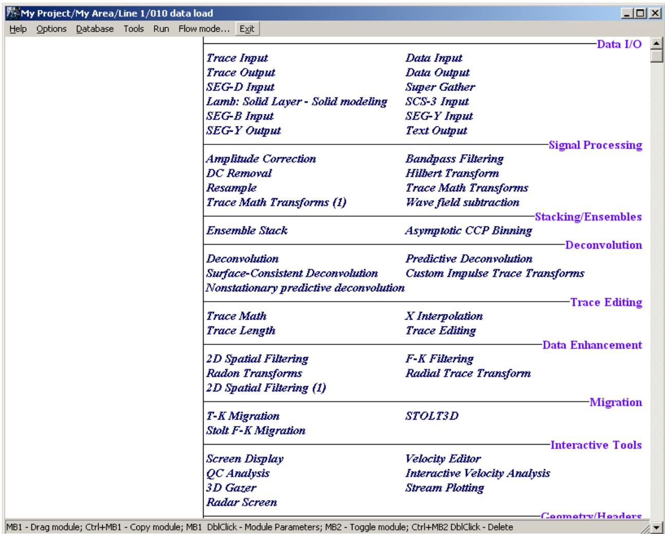
Create a flow, consisting of the modules **SEG-Y Input** and **Trace Output** (both are located in group **Data I/O**). This flow will read the data from a SEG-Y- file and record them into the project database a "dataset"-object of the database..
