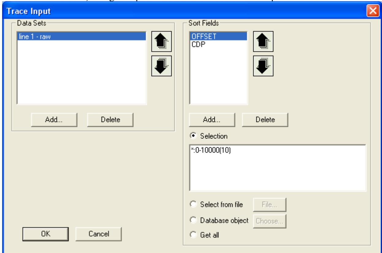
Execute the flow; the traces, sorted out in ascending order of the OFFSET header field will be shown on the screen. Such a gather (called, common-offset gather) allows convenient assigning the muting time, which will be suitable for all CDP gathers.
