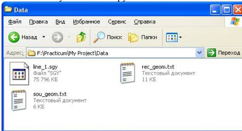
Storing the data inside the folder of the project allows the software to use relative paths to the data files instead of the absolute ones. This makes the transfer of projects from one computer to another much easier.
