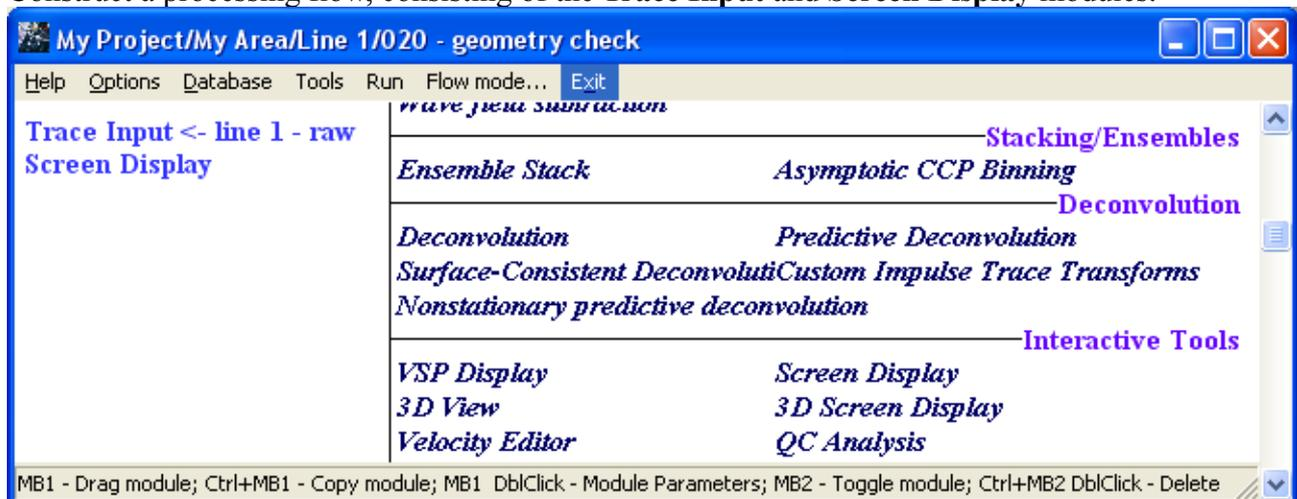
The **Trace Input** should enter the data into the flow sorted by, primarily, CDP and, secondarily, OFFSET (hereinafter, we will use CDP:OFFSET notation to describe this sorting). For this, set the routine parameters as shown on the following figure.
