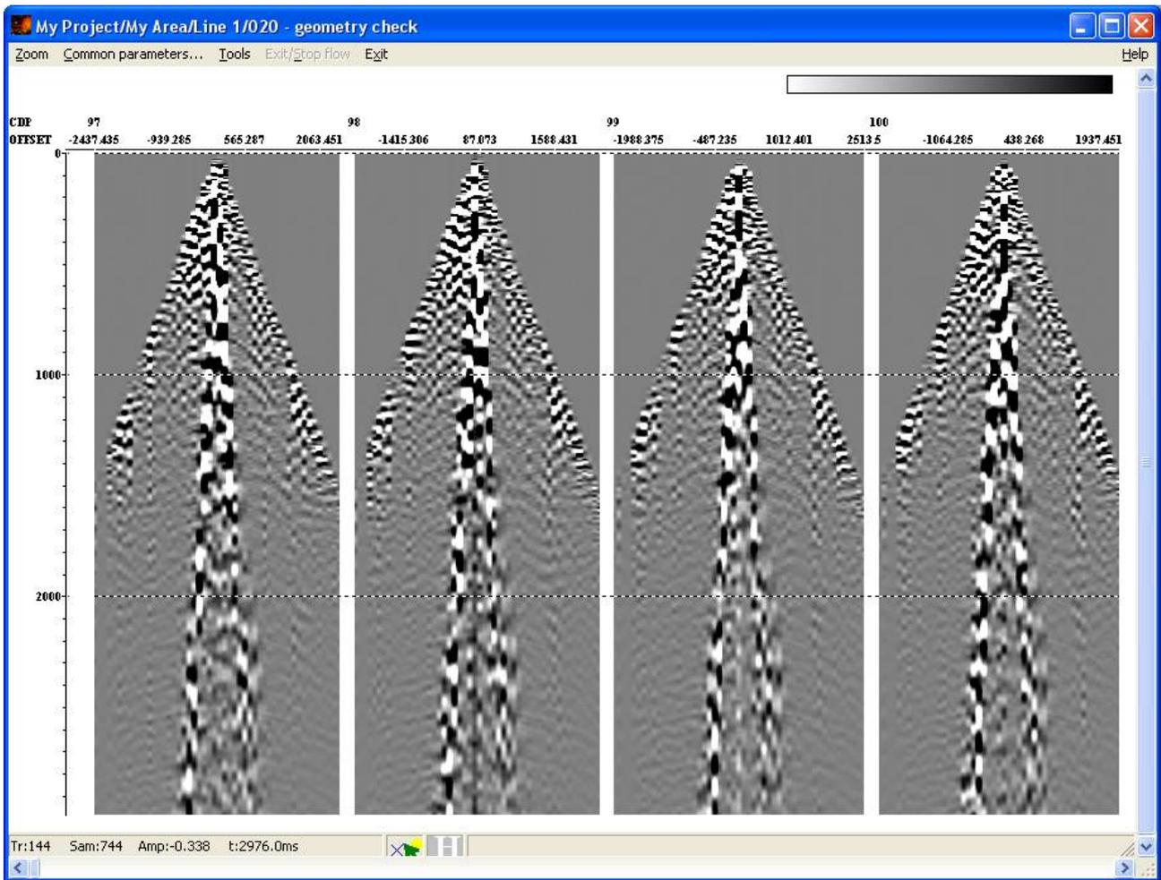
To control geometry assigning display the theoretical travel times of reflected wave calculated from header field values. To do it use the **Tools/Approximate/Hyperbola (reflection)** entry of the **Screen Display** menu.
