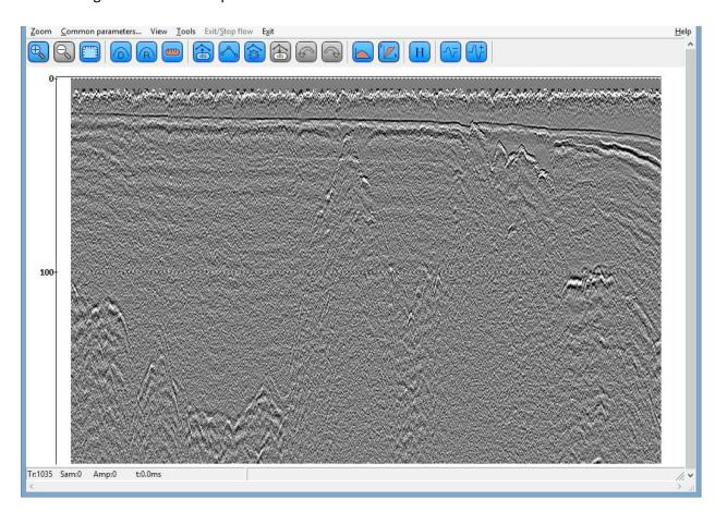
A result of F-K Amplitude Power algorithm applied in sliding windows:
