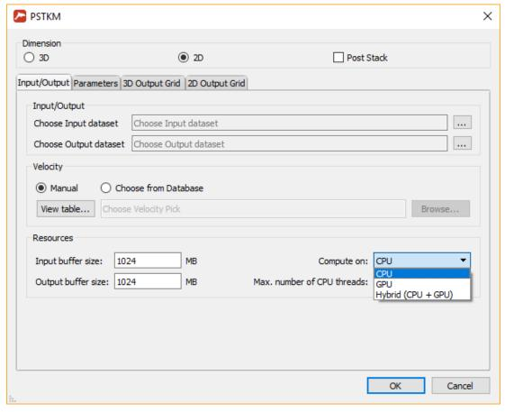
We recommend that only those GPU that are not connected to a display shall be used for calculations. The module would automatically select the most powerful GPU from those available.
