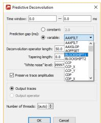
Predictive Deconvolution can now use variable gap taken from trace header.
