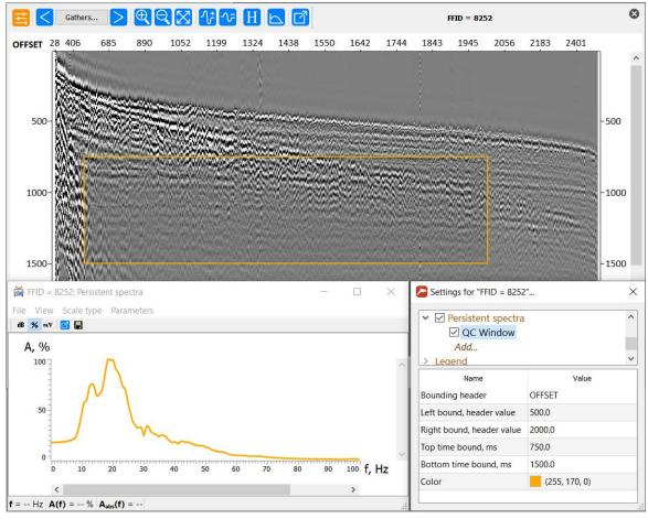
• In the seismic display window of the **Interactive QC** module, now you can filter the list of gathers to display using an arbitrary header, as well as search for a particular gather in the list.
