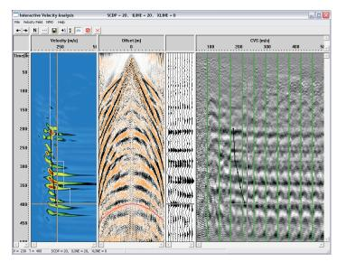
The data display module supports all types of display and easily synchronizes scale, position, and gain between several windows for convenient comparison of processing results.
